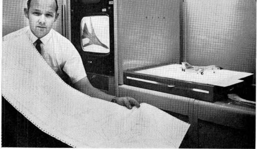
DATA REDUCTION of graphic materials has been made considerably cheaper through development of the Sandia Image Digitizer-II. Developer Bob Cover (1724) displays the computer readout version of an F-111 model aircraft. The F-111 model is viewed by a TV camera (right), reproduced in analog form (lower TV screen), converted to digital outline (upper screen) and then relayed to a computer for analysis, simulation, or other programmed treatment.
